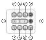
1. "ON" KEY: Press to turn on the scale.
